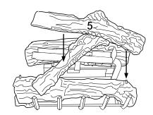
Figure 49 - Installing Log No. 5
